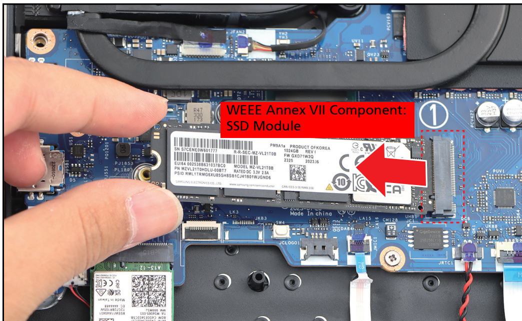
Figure 1-10. Removing the SSD 1 Module
