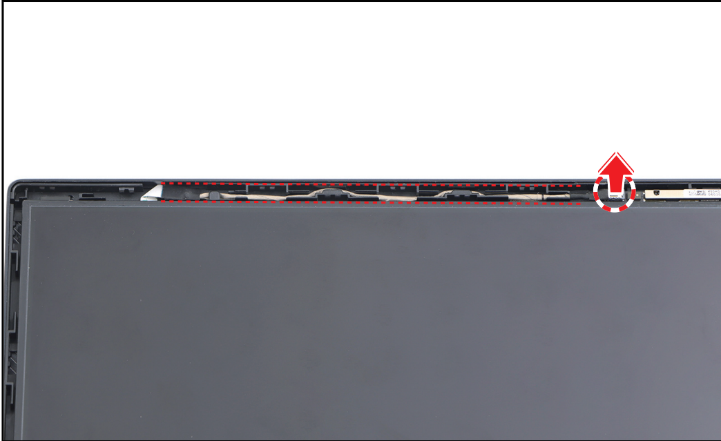
Figure 1-50. Disconnecting and Unrouting the eDP Cable
