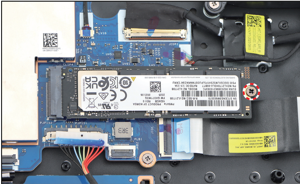
Figure 1-11. Removing the Screw
