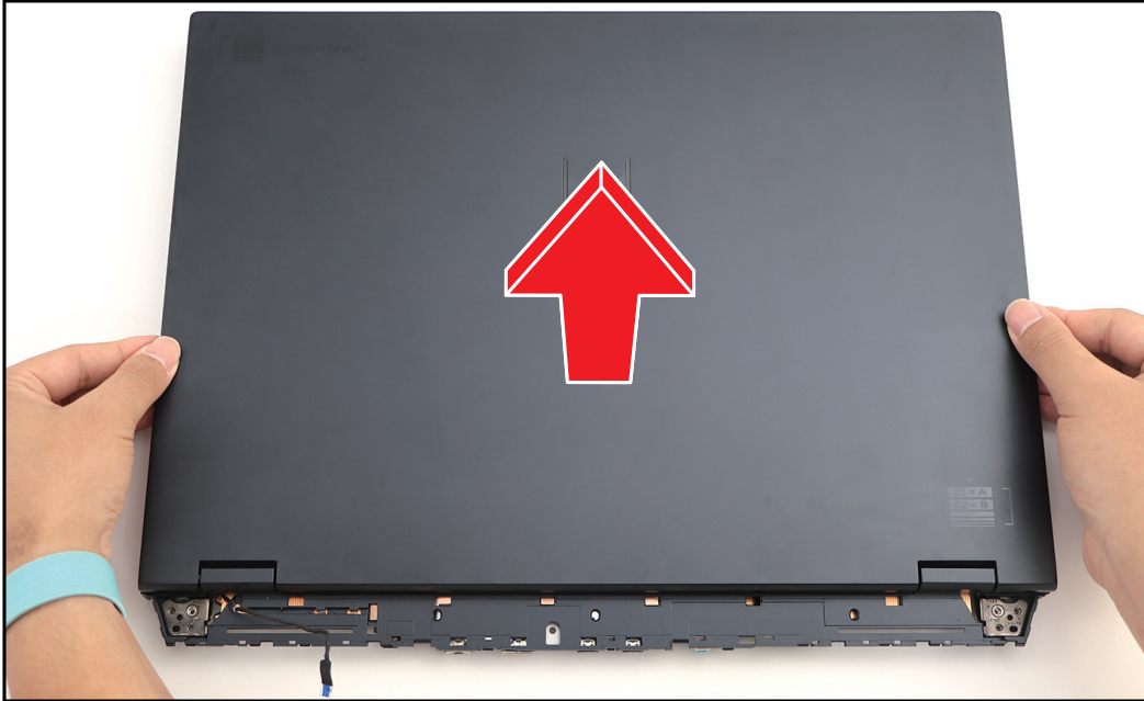
Figure 1-30. Releasing the LCD Module
