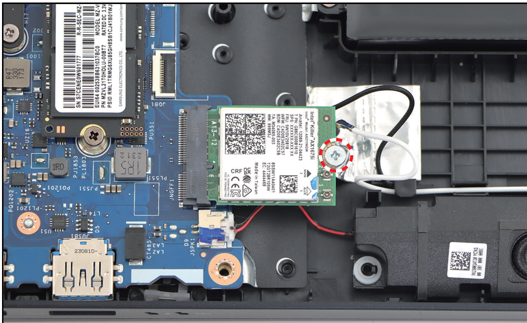
Figure 1-14. Removing the Screw
