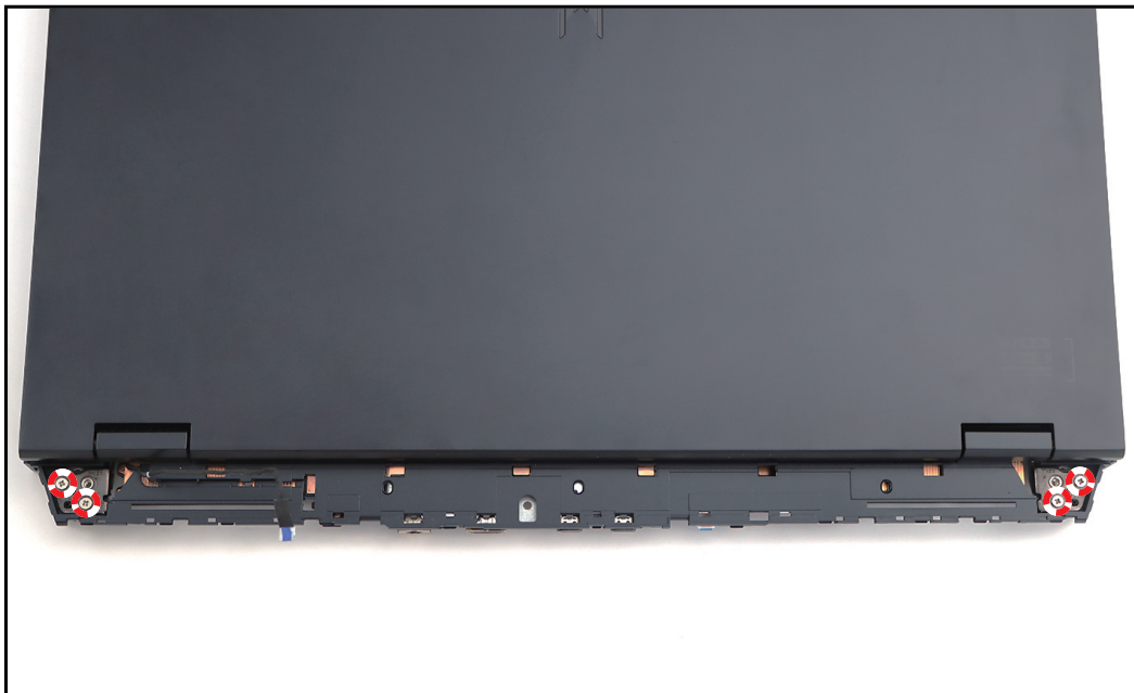
Figure 1-29. Removing the Screws
