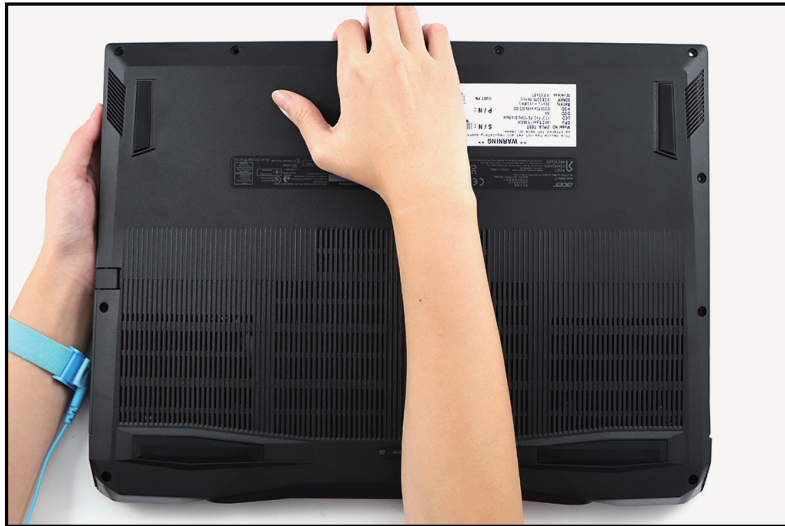
Figure 1-5. Base Cover Removal
