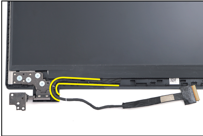
Figure 1-51. LCD Panel Removal
