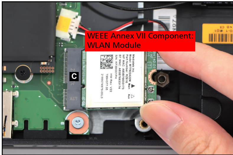
Figure 1-30. WLAN Module Removal
