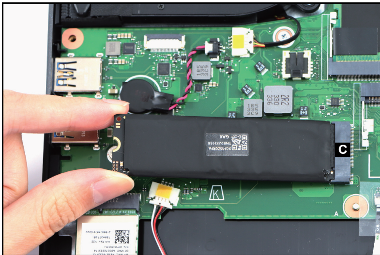
Figure 1-18. SSD Module Removal
