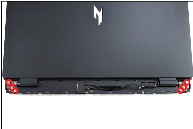
Figure 1-46. LCD Module Removal
