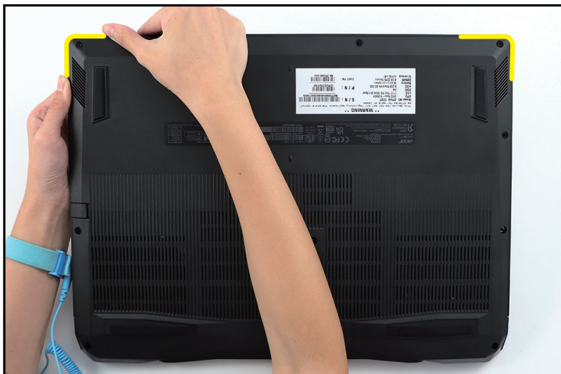
Figure 1-4. Base Cover Removal
