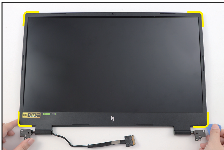
Figure 1-50. LCD Bezel Removal
