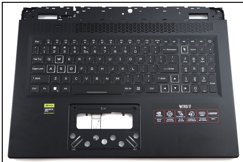
Figure 1-56. Top Assembly (Keyboard)
