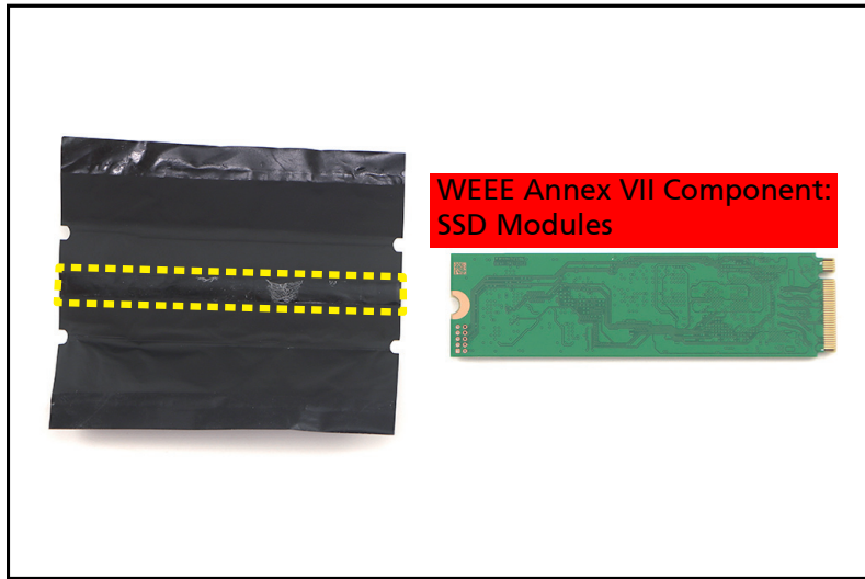
Figure 1-21. SSD Module Removal
