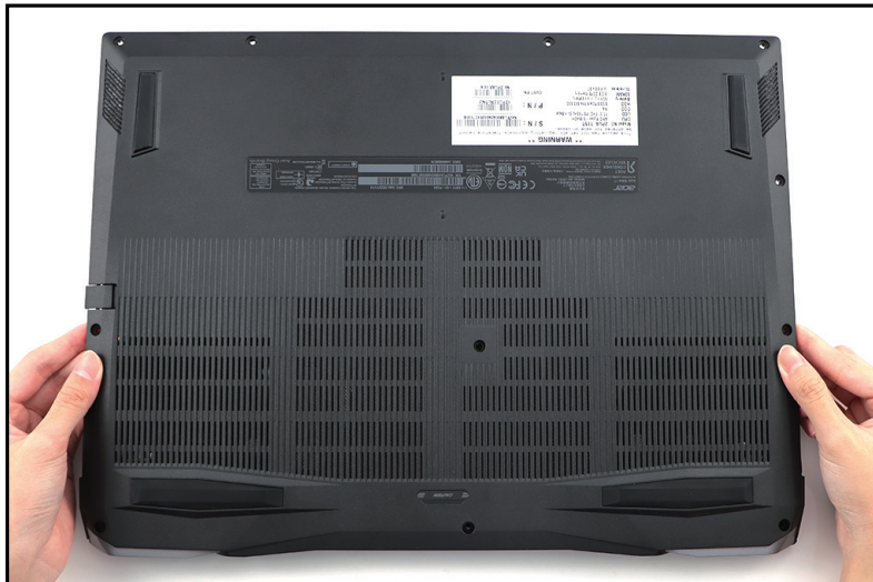
Figure 1-6. Base Cover Removal
