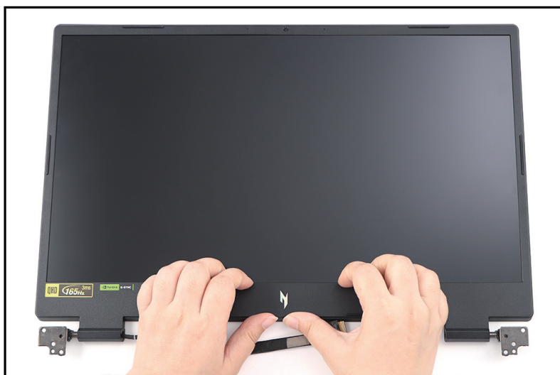
Figure 1-48. LCD Bezel Removal
