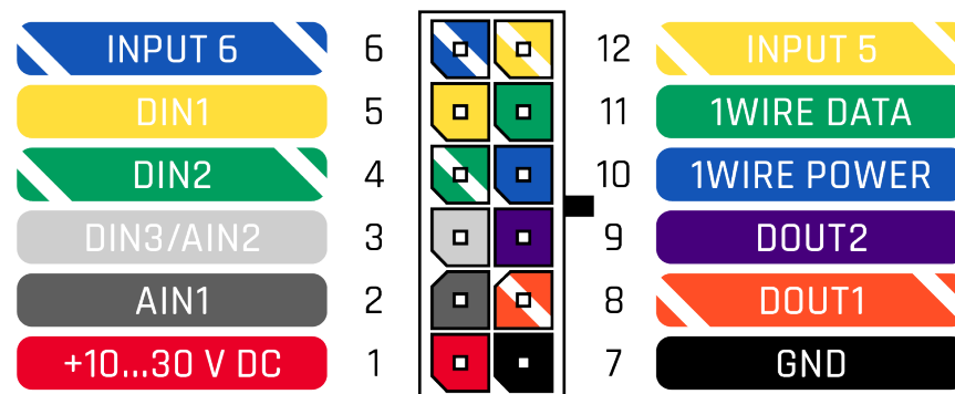
Figure 2 FMB120 2x6 socket pinout
