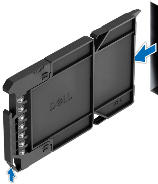
Figure 76. Removing an EDSFF E3.S drive blank
