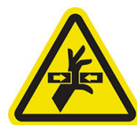
Hazardous moving part
