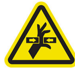
Hazardous moving part
